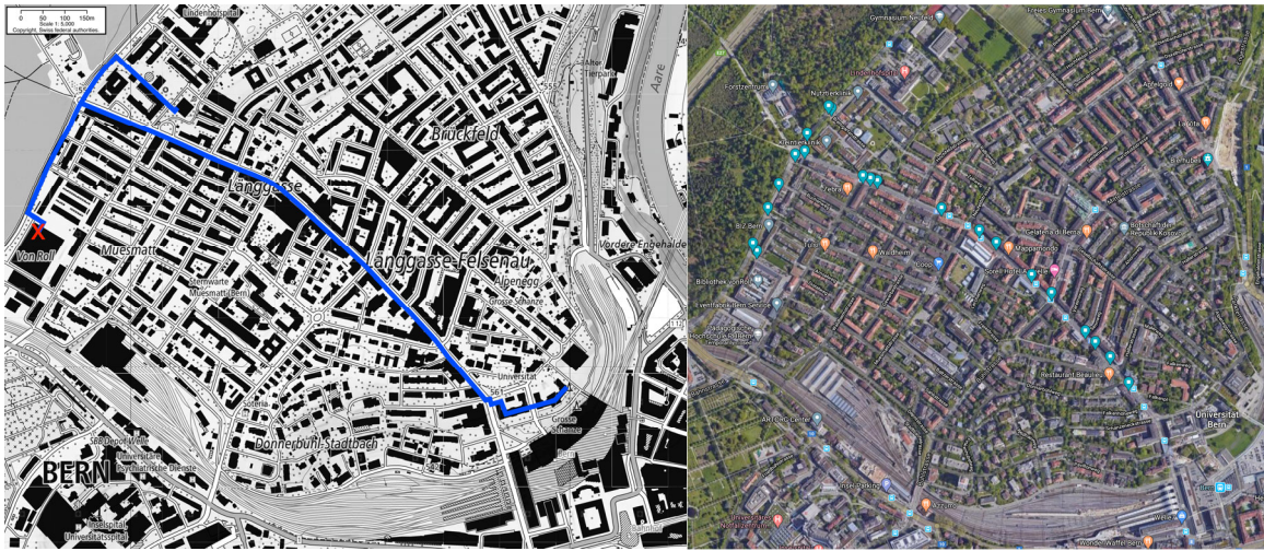
Figure 1: (a): The blue line shows the location of the fibre beneath Bern, Switzerland. The red cross indicates the position of the iDAS interrogator (b): The collected GPS points used for calibration of the fibre data with physical locations
