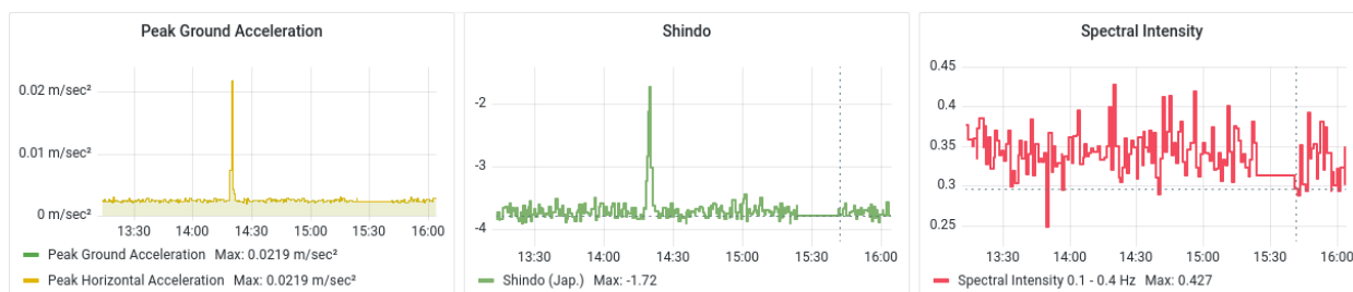
Figure 7: Real-time ground monitoring from the Montenegro network showing calculated peak ground acceleration, Japanese intensity measure (Shino) and spectral acceleration.
