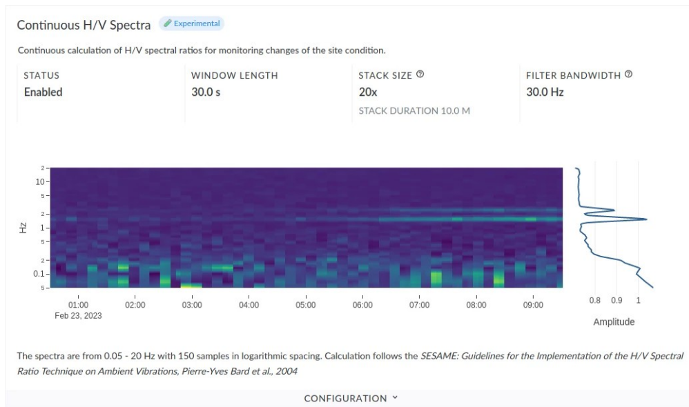
Figure 8: Continuous H/V spectra delivered by a QuakeSaver MEMS sensors installed in a 13 storey building by RISE partners in Switzerland. Clear Eigenfrequency modes of the building are visible in the delivered data.
