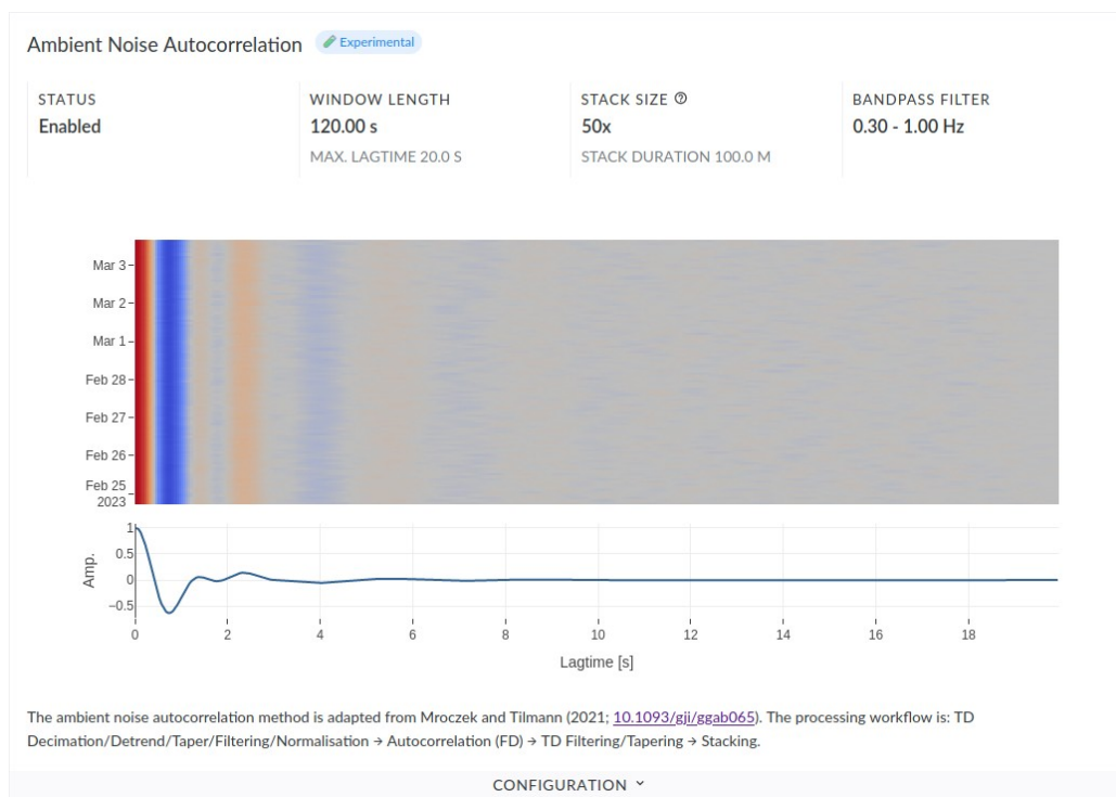
Figure 9: Noise autocorrelations calculated on the QuakeSaver sensor deployed by RISE partners in Montenegro.
